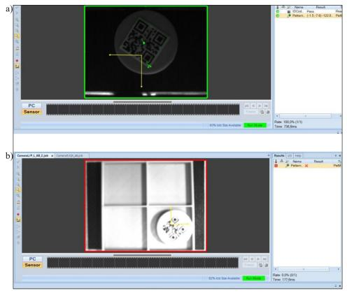
Fig. 4. Screens from RobotStudio software connected with Integrated Vision in SmartGripper by (a) underexposure, (b) overexposure
