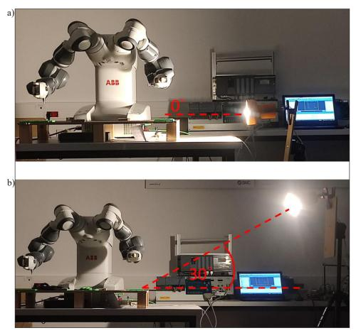
Fig. 6. Experiment with different angle of incidence (a) 0°, (b) 30°
