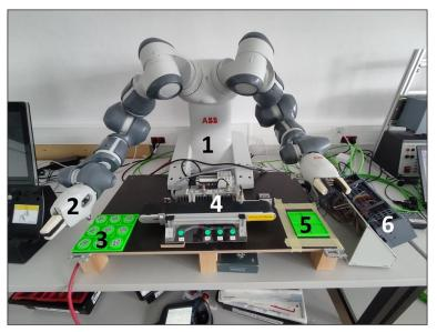
**Fig. 1.** Collaborative robot YuMi IRB 14000 used in the experiment. In Figure, the most important elements are marked, i.e. 1 – collaborative robot ABB IRB 14000 YuMi, 2 – vision system in the robot arm, 3 – place plate with elements, 4 – conveyor belt, 5 – pick plate, 6 – PLC controller
