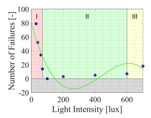
**Fig. 5.** Number of failures of vision system in the domain of variable angle of incidence. Green curved line corresponds to the cubic fitting to the results obtain of number of failures
