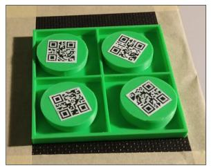
Fig. 3. 3D printed elements with QR codes used in the experiment
